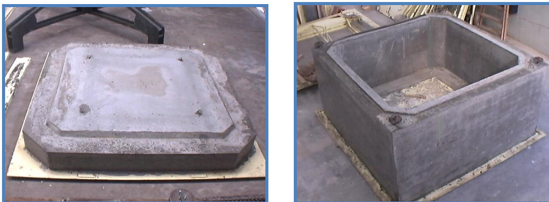
Figure 2.3 INTI's Prototype container originally designed for radioactive waste
